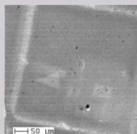
SEM micrographs of U<sub>3</sub>O<sub>8</sub> particles from SRM-U900
